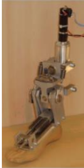
Figure 14. Tethered prosthesis developed by Carnegie Mellon University, USA [3]
